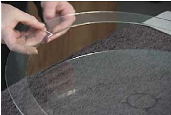
If you measured right, the rim will fit perfectly around your interior design at project layup. The single seam will heal during the firing process and be undetectable in the finished piece.
