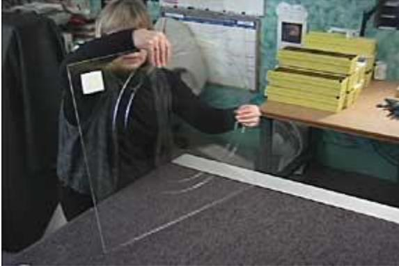
Make relief scores, drawing your glass cutter outward from the outermost circle score to the edge of the sheet. After making one, **rotate the sheet without lifting it**, to prevent it from collapsing under its own weight.
