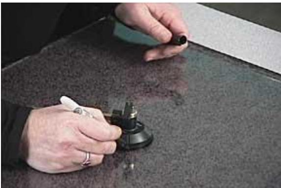
Patty oils the cutter-head before scoring. She uses an oil-soaked cloth placed in a jar lid.
