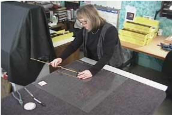
Once the circle-cutter is properly positioned, she marks the center for future reference. (Knowing the center position can come in handy later).
