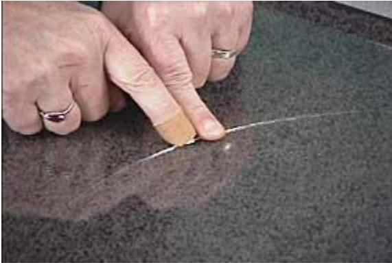
Remember to press gently. Smaller circles require more pressure, because the glass doesn't flex as easily. Seek to "run" the score completely around your circle or oval. Go over the score line a few times, all the way around, until you are satisfied the "run" is complete.
