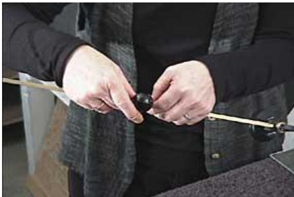
You'll score the inside of the rim first, so position your circle-cutter center, taking care to ensure that there is space enough to accommodate both the width of your border and 1/2" (12mm) clearance from the edges of the sheet. Example: if you are cutting a border 1 1/2-inches (4 cm) wide, you'll need at least 2-inches (5 cm) of clearance to the sheet edge, on all sides, for the first score.
