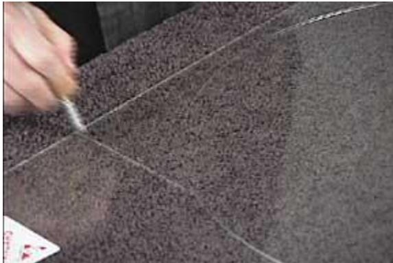
Then, run each relief score using a method or tool with which you are comfortable.
