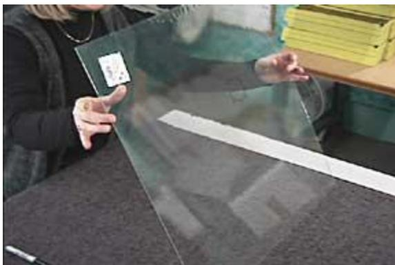
Then she applies pressure directly to the back side of the score. In transparent glasses, you can see the score propagate, or "run" along its path. In opal, or denser glasses, you can see a "dimpling" occur as the score runs its course.
