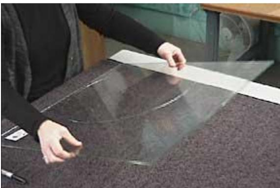
Next, make "relief" scores in the four corners of your square sheet. Rotate the sheet flat on the table, without lifting it, to position it for making the relief scores. The sheet weakens with each score, and could break apart at any time.
