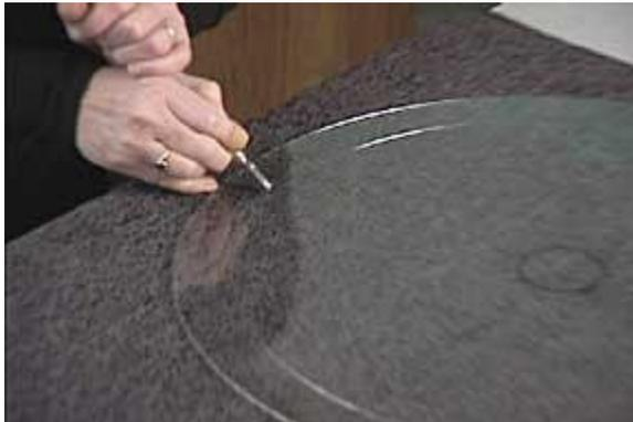
This relief score releases tension in the border "donut" and allows it to be separated cleanly from the inside.
