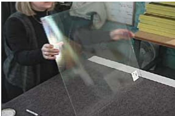
Now begin running the scores by applying gentle pressure to the back side of glass, (as explained in the circle-cutting demonstration).
