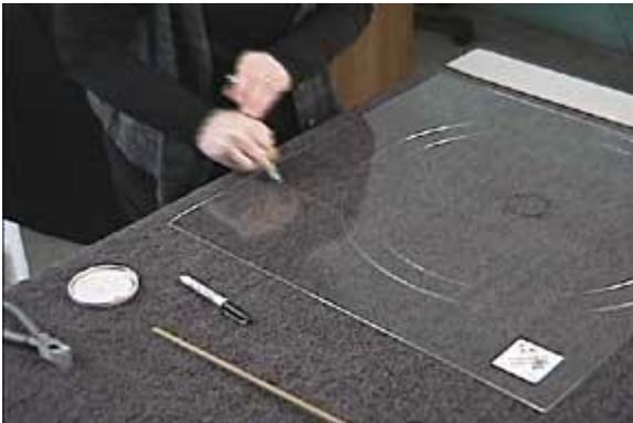
Run the relief scores one at a time; again, rotating the sheet *flat on the table*. **Do not lift the sheet.**
