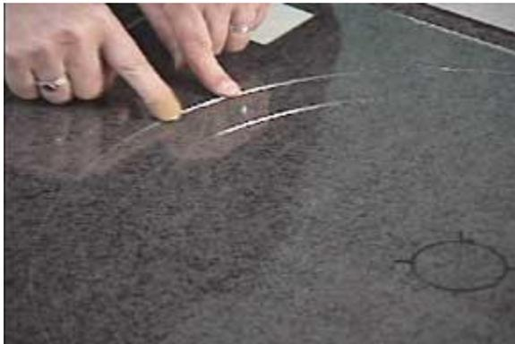
Apply pressure all the way around both scores a few times, until you are satisfied that both scores are fully propagated. If the glass is not transparent, make sure you are pressing exactly on the backside of the score, and watch for slight dimpling or other indicators that the score is running.
