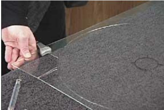
As the relief scores are run, the sheet edges should fall easily away from the circle.
