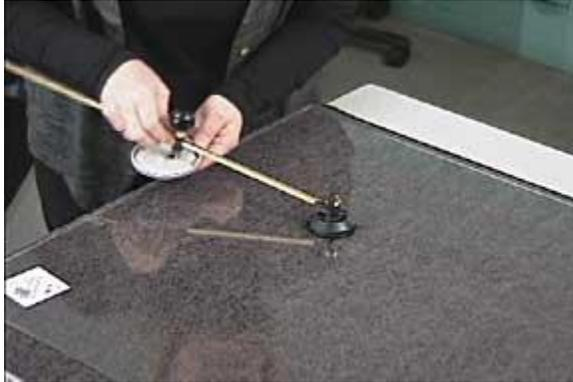
She rotates the cutter-arm, scoring the glass 360 degrees in a smooth motion with even pressure. Then, she removes the circle-cutter from the glass
