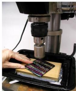
Before you begin coring you will need to get some idea of **WHERE** you want to make your first cut. While holding the glass firmly against the wood block, you will gently lower the pilot feed lever until the drill bit makes contact with the
