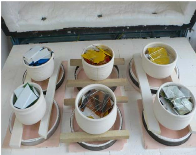
This photo is taken in my top loading Genesis kiln. I have each pot melt set up on a small kiln shelf only because my larger shelf was not dry at this moment.....These small shelves are sitting right on the kiln brick. As you can see I pile the glass high. Personally I use a lot of opaques and whites mixed in. Be sure to take notes on every load. I use
